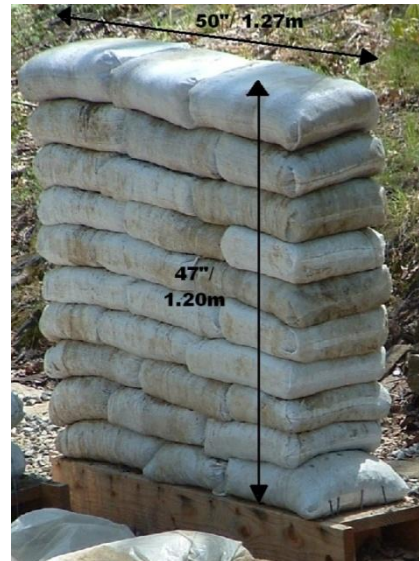
Right above: Before and after tamping Right: Finished test wall
