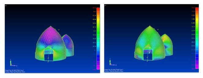
Figure 4: Maximum shear stress
