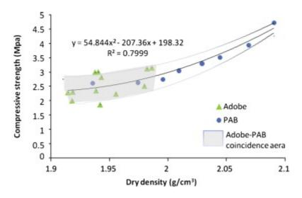
Figure 6: Relationship between ovens dried density and compressive strength (Kouakou 2009)
