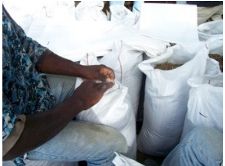
The bags were sewn shut with wire. Poking the wire through the bags 5 times (14" wide bag) seemed to be adequate and fast. Cutting the wire at an angle definitely aided in penetrating the sacks.
